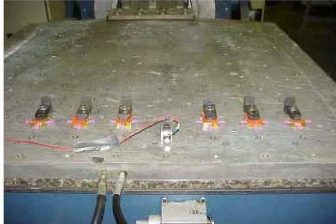
Figure 2-3. Test setup for longitudinal-axis Willoughby random vibration.
