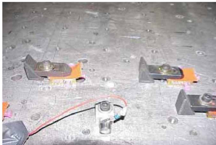
Figure 2-4. Test setup for lateral-axis Willoughby random vibration.
