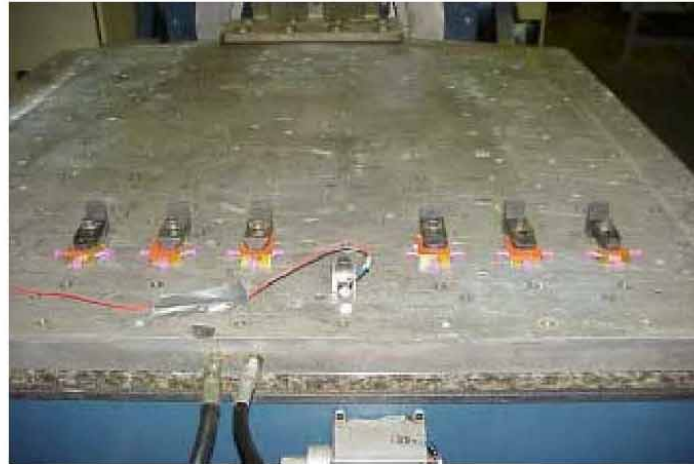
Figure 2-3. Test setup for longitudinal-axis bulkhead mounted level MPE random vibration.
