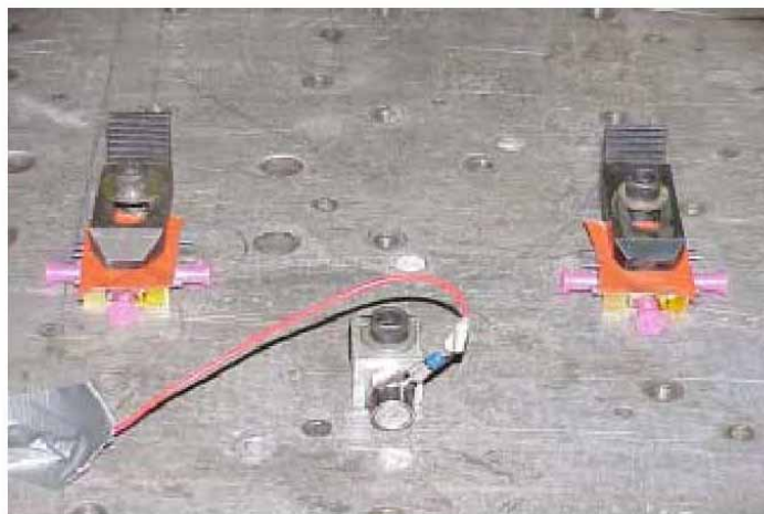
Figure 2-2. Test setup for longitudinal-axis Willoughby random vibration.
