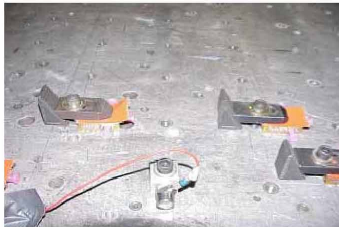
Figure 2-4. Test setup for lateral-axis bulkhead mounted level MPE random vibration.
